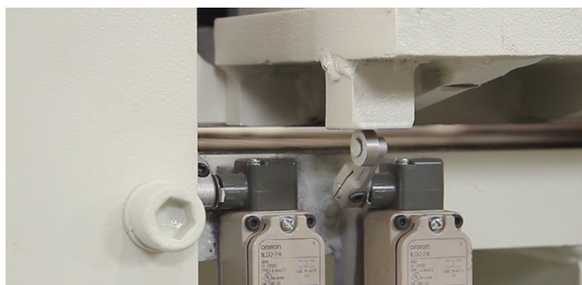
Moving bolster is not reached read limit switch
